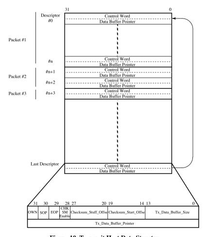
Figure 10. Transmit Host Data Structures
